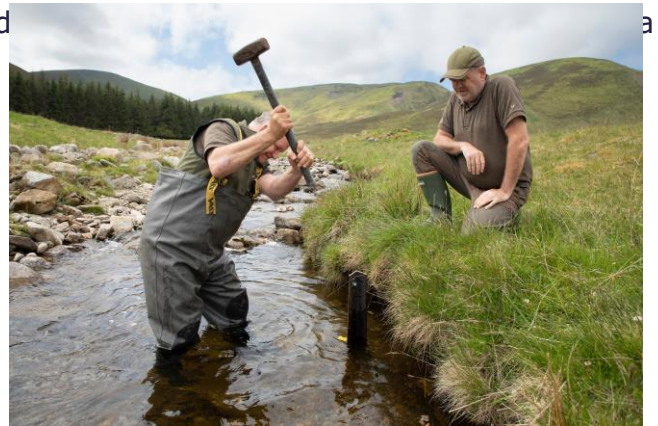
Hard graft! Sean Mclean and Alister Taylor installing a temperature monitor. (photo ScotlandBigPicture )
